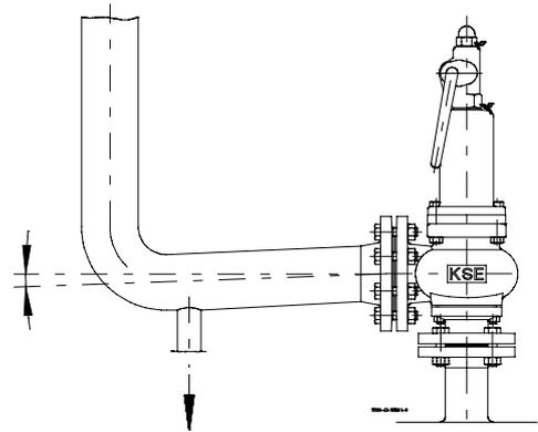
Lines for the drainage of condensate are to have adequate cross sections. They are to be laid with a gradient and must ensure safe drainage of the medium.
