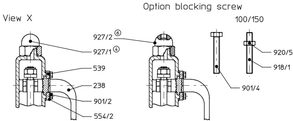
⑥ Cap nut 527/2 with a additional tapped bore for blocking screw. The threaded rod 918/1 for size 100/150 is screwed directly into the lifting cap 535.
