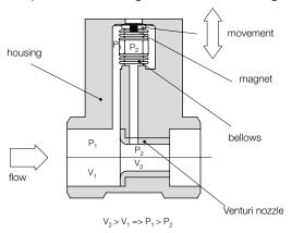
If the flow is exceeded the differential pressure measuring cell is protected by locking pins. On mechanical displays the flow rate measured by the pressure measuring cell is transferred via a pointer movement to the pointer indicator calibrated in l/min water or Nm³/h air. On electronic displays the mechanical motion is converted to an electrical signal by a Hall-sensor. Various electronic modules are then used to display and monitor the volumetric flow.
