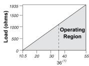
Power Supply Output Code S (dc Volts)
