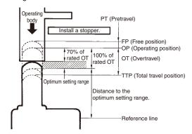
The Limit Switch may soon malfunction if the OT is excessive.
