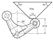
Note: Design the shape of the dog so that it does not come in contact with the other roller lever when the actuator is inverted.
