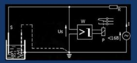
When the electrode and liquid come into contact (resistance R c decreases accordingly ), electric current begins to flow in the circuit: current source, matching resistor R (range), connecting wire, electrode S, conductive liquid, conductive tank wall or additional electrode for a non-conductive tank, and a second connecting wire. The control signal U decreases, and the relay system is activated.
