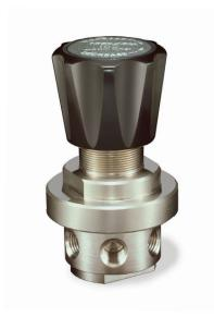
TESCOM 44-2600 Series is a compact, extremely sensitive, high purity single-stage regulator for specialty, flammable and industrial gases with flows of less than 10 SCFM / 283 SLPM. Diffusion-resistant metal diaphragm seal ensures gas purity and integrity.
