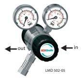
Dual-stage, for inert, reactive, flammable and oxidizing gases and gas mixtures, purity max. 6.0 inlet pressure 230 bar / 3300 psi, downstream pressure range 0.2 - 10.5 bar / 3 - 150 psi
