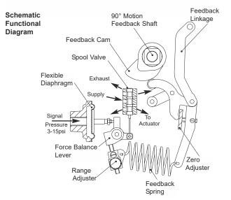
The AP positioner moves an actuator to a position set by a 3-15psi control signal and holds it there. Its features are:
