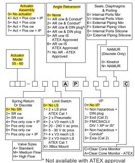
'A' Valve is supplied with all sizes up to and inc' 09 'M' Valve is supplied with 10-15 'H' Valve is supplied with sizes 16-60
