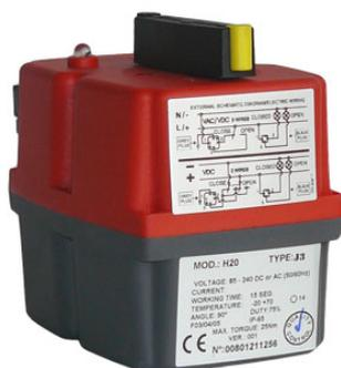
Protection against valve jams is provided by an electronic torque limiter, which auto-relaxes the gearbox when activated, allowing the manual override to be selected to assist in clearing the jam.
