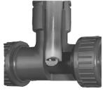
When liquid flows through the pipe, the paddle wheel with 4 inserted magnets is set in rotation, producing a measuring signal in the sensor (Hall sensor). The frequency modulated induced voltage is proportional to the flow velocity of the fluid.
