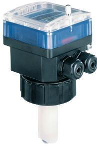
The compact batch controller combines a paddle-wheel flow sensor and an electronic module with a display in an IP65 enclosure. The electrical connection is provided via two cable glands.
