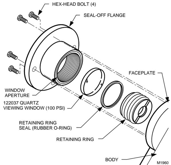
**Fig. 23. Replacing quartz viewing window on C7012C,F.**
