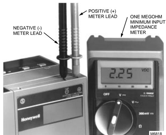
Fig. 19. Measuring voltage flame signal with 7800 SERIES controls.
