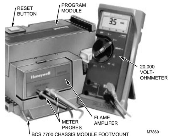
Fig. 18. Measuring voltage flame signal with BCS 7700 controls.
