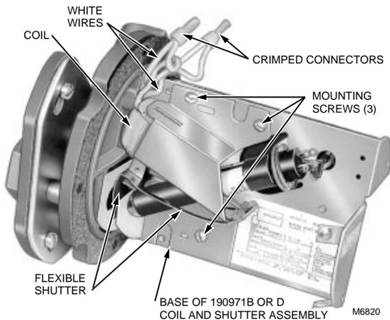
**Fig. 21. Replacing coil and shutter assembly on C7012E,F.**
