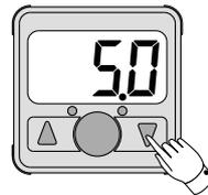
Press the ▲ button at least for 1 second during pressure display to enter the bottom display mode. The displayed value will blink. To return, press the ▼ button again at least for 1 second.
