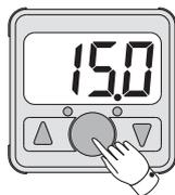
Select the manual setting mode as the initial setting mode. Press the SET button and hold it until "P\_1" or "n\_1" appears on the display.
