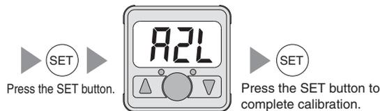
Repeat vacuum and break several times while "A1L" is displayed. The optimum set point value is determined automatically.
