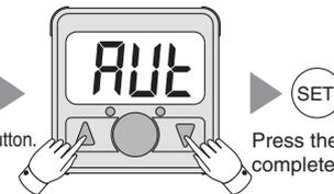
Select the auto preset mode or manual calibration mode with the ▲ or ▼ button.
