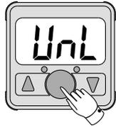
Press the SET button at least 2 seconds. Release it when the display turns to "UnL".
