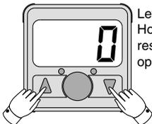
Let the supply pressure open to the atmosphere. Hold both ▲ and ▼ buttons simultaneously to reset the display value to zero. After resetting, the operation returns to the measurement mode.
