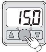
Select auto preset mode as the initial setting mode. Press the SET button and hold it until "RP1" appears on the display.
