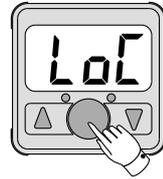
Press the SET button at least 4 seconds. Release it when the display turns to "LoC".
