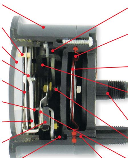
**Range spring calibration clamp** fixes live length of spring for proper gage calibration and is factory set and sealed.
