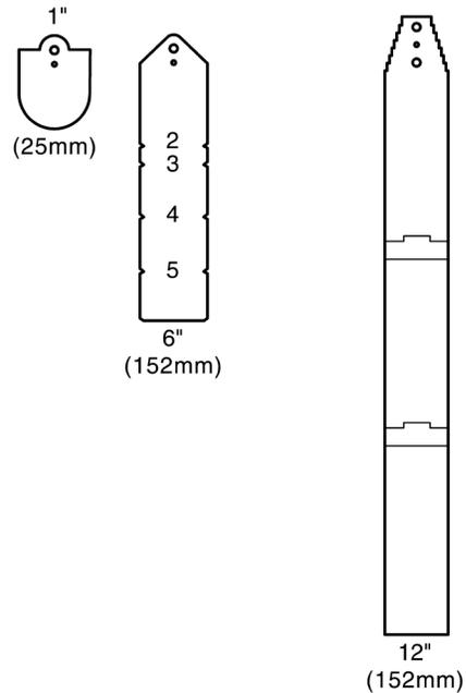
a. Trim paddle by cutting at appropriate notch with non-serrated tin snips.
