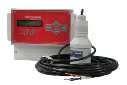
The SONDAR SLM800S, 1200S and 1500S are a highly developed ultrasonic level measurement system, which provides in non contacting level measurement for a wide variety of applications in liquid and solid. The SLM1000 Series consists of a micro-processor based controller and sensors that can be mounted up to 8m, 12m and 15m respectively according to field requirement.
